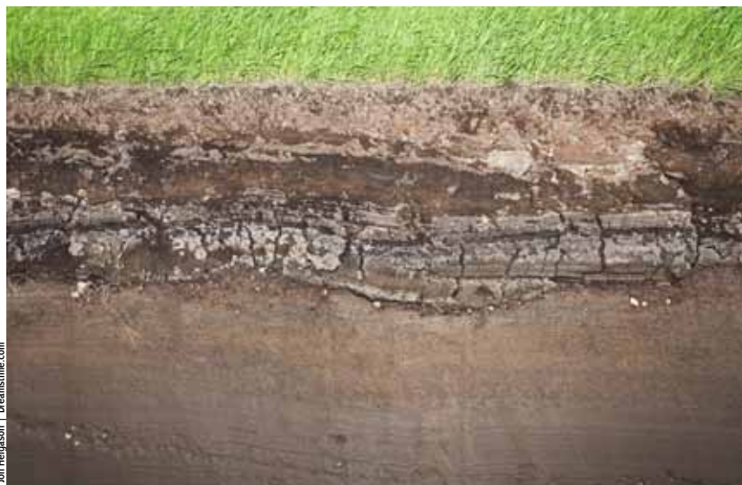
The soil under a thin layer of topsoil and grass can become compacted, stopping rainwater from infiltrating, so stormwater, nutrients, and pesticides are more likely to run off.
